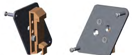
DIN rail mount adaptor for CT electronics
